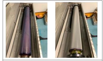
Image of an anilox roller: left before cleaning, right after cleaning with Böttcherin Solvento (application in the automatic washing system)
