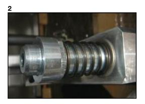
1 Drive spindle → pivot center for Heidelberger (for other presses pivot center is different)
