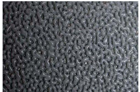
Image: surface of a stochastically laser engraved film roller
