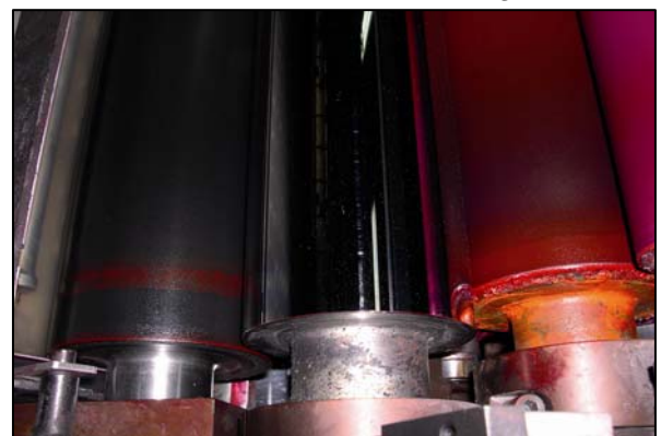
Fig. 2: Ink feedback onto the dampening pan roller (left)
